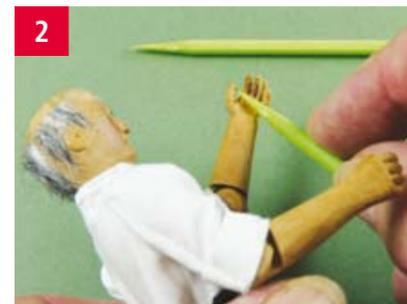
Plastic Sanding Needles, a 3/16in diameter rigid plastic file with a sharp point at one end and an oblique cut at the other end with various grits bonded to the surface, again conveniently colour coded. Ideal for smoothing all those intricate corners and confined spaces.
