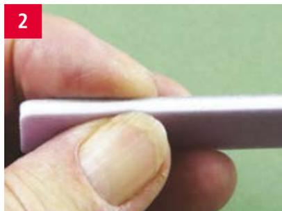
The Sanding Files have the same rigid foam core, which is soft enough to squeeze. Each side of a file is coated with a different abrasive grit and with its own coded colour. ■ Sanding works by scratching the surface, each grade in turn puts in finer scratches. The object has a perfect finish when the scratches are so fine that they cannot be seen.
