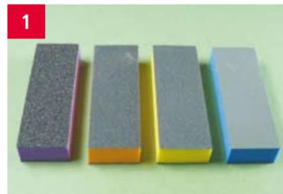
Super Sanding and Finishing Foam Block, is a long title for a very useful basic sanding system. ■ Each block has a different grit on each side, bonded to a soft foam core. If a piece of wood requires sanding and all eight grits are used in turn then a perfect finish will be obtained. It is important only to work along the grain of the wood. The sanding blocks are also suitable for plastics and metals, even though these have no grain, try to work only in one direction to gain the best finish.
