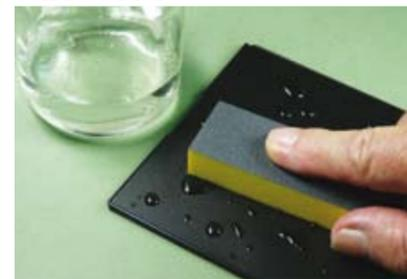
All Crafty Cat products can be used wet, that is with a little water added to the surface. ■ Can be a little messy! Can only be used on surfaces not harmed by water, so do not use on bare wood.
