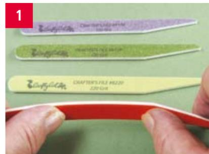
The Crafter's File has a plastic foam core that is sufficiently rigid to work with one hand but flexible enough to be used in awkward corners. ■ The files come ready shaped with a taper and a rounded point, but could be trimmed to any convenient shape. Both sides of the file are coated with the same abrasive grit and coloured for quick recognition for the grade required.
