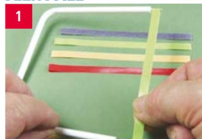
Flex-I-File, is a unique system for smoothing and polishing curved surfaces. It consists of a slightly sprung aluminium bow frame with a prong at both ends. It comes with strong flexible abrasive tapes that have a loop at each end. These loops are hooked over the prongs.
