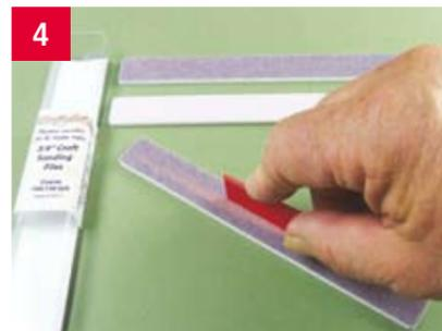
To smooth a straight edge and to keep it at 90°, it is easier to place a file on a flat surface and move the object backwards and forwards. Do not put on any downward pressure as it will sink slightly into the foam and give a rounded edge.
