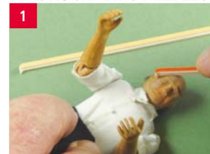
The fine sanding files are excellent at smoothing intricate shapes, here being used on a doll's head. ■ The resin heads of scale figures, which have been cast in two part moulds, often have a tiny ridge where the halves meet (often called a flash). This needs smoothing away without scratching the surface, a job for Crafty Cat sanding files!
