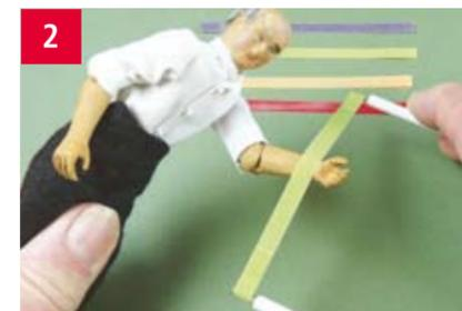
The Flex-I-File is squeezed gently to give the tape some slack so that it follows the contour of the items to be smoothed. Try to use the full length of the tape to even out the wear.
